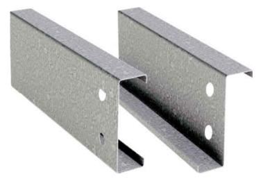
Purlin, commonly termed as Z and C Sections, are defined by a central vertical web joined to horizontal flanges at either end. Additional lips are included to support the flanges. It is available in HR and GI grades and also in different thicknesses and depth depending on design of the building. Purlin can be supplied in customized length with pre-punched holes as per architectural designs.
